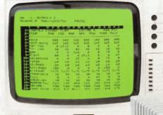
The high resolution display of 256 x 192 pixels is retained and all the currently available Dragon data software both on plug-in cartridge and cassette will run on the 64.
